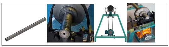
Figure 12: Shaft connected for balancing.
