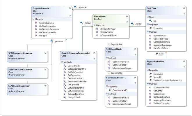
Figure 4 - Class Diagram of SEA Constraint Language Code Generator.
