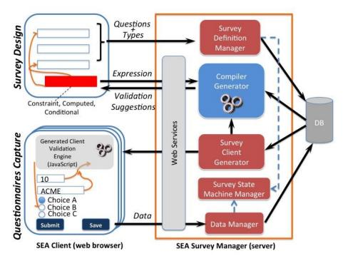
Figure 1 - Architecture of the SEA Platform.
