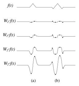
**Figure 2** - ECG scheme and some of its dyadic wavelet transforms. Dots represent the modulus maximum. (a) P-, T- or U-wave scheme. (b) QRS complex scheme.
