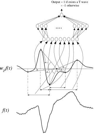
Figure 3 - T wave maximum point detection scheme.
