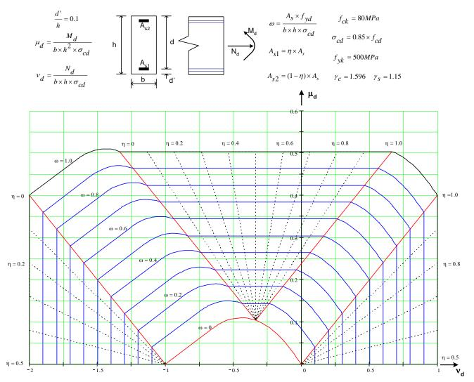
**Figure 10** – Design axial load and moment interaction chart for HPC with d'/h=0.10 and  $f_{ck}=80$  MPa – CEB Bulletin d'Information No 228.
