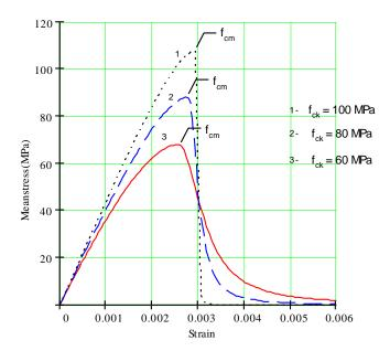
Figure 2 – Realistic curves of 3 different types of HPC for uniaxial compression and short term loads considering the mean compressive strength and showing the entire descending branch.
