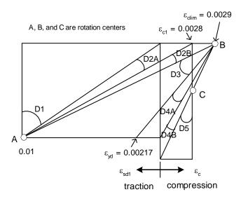
Figure 5 – Reinforced concrete strain domains with  $f_{ck}$ =80 MPa and  $f_{vk}$ =500 MPa.
