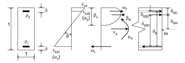
Figure 4 – Stresses and strains diagrams showing the reduced parameters.
