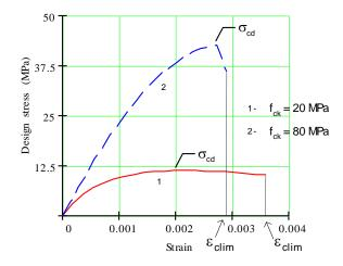
Figura 1 – Design stress-strain curves of a HPC and a conventional concrete.
