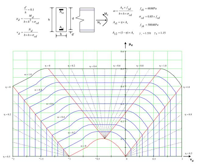
**Figure 8** – Design axial load and moment interaction chart for HPC with d'/h=0.10 and fck=60 MPa – CEB Bulletin d'Information No 228.
