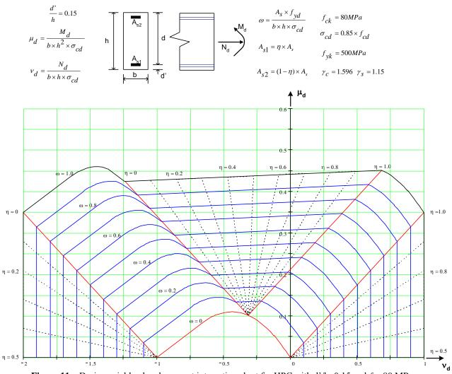
Figure 11 – Design axial load and moment interaction chart for HPC with d'/h=0.15 and  $f_{ck}$ =80 MPa – CEB Bulletin d'Information No 228.
