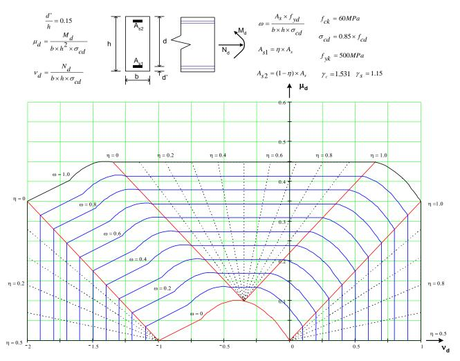
**Figure 9** – Design axial load and moment interaction chart for HPC with d'/h=0.15 and  $f_{ck}$ =60 MPa – CEB Bulletin d'Information No 228.
