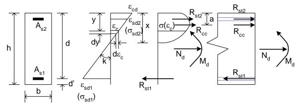
Figure 3 – Stresses and strains diagrams.
