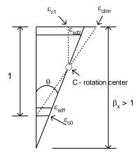
Figure 6 – Failure strain configuration of the domain D5.
