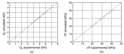
Figure 3 - Comparison of simulated with experimental results in terms of: (a) heat rejection rate; (b) refrigerant pressure drop. Refrigerant: HFC-134a; inlet air temperature: 40°C; refrigerant mass flow rate: 0.0198 to 0.0335 kg/s; inlet temperature of the refrigerant: 70.2 to 94.4°C; saturation temperature of the refrigerant at inlet pressure: 49.2 to 56.7°C.
