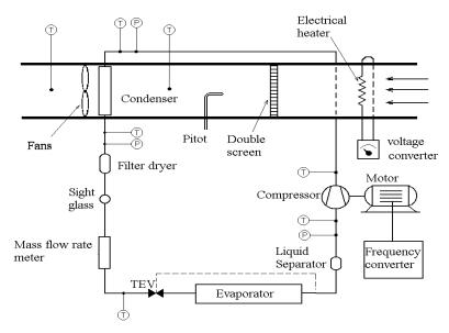
Figure 2 - Schematic diagram of the experimental bench.
