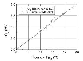
**Figure 4** -  $Q_{cond}$  vs  $[T_{cond} - (T_a)_{in}]$ . Refrigerant: HFC-134a; inlet air temperature: 40°C. Same ranges of other input parameters as in Figure 3.
