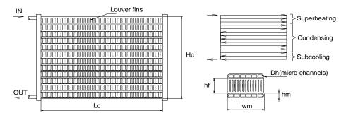
Figure 1 - Schematic representation of parallel flux micro channels condenser.
