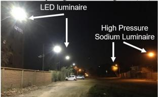
Figure 16: The complete deployed pilot system, comparing LED luminaires and High-Pressure Sodium luminaires.
