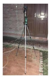
Figure 17: Luxometer on tripod.
