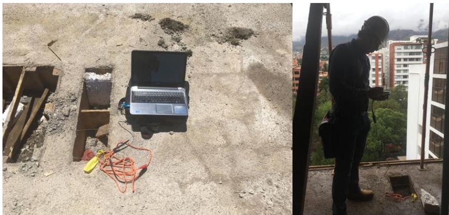
**Figure 8: Slab Maturity Index Readings.**
