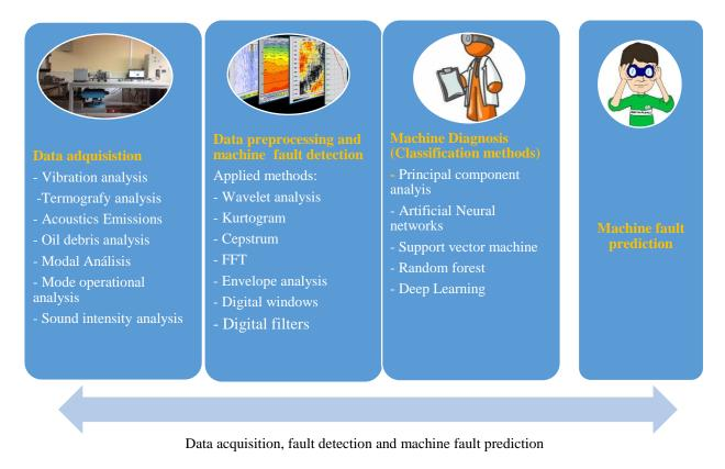
Figure 1- The flowchart of the machine diagnostics. a) Data acquisition , b) Fault detection , c) Fault classification , d) Fault prognosis.
