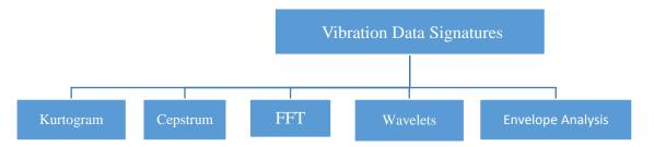
Figure 8 - Different methods for Vibration based fault detection.
