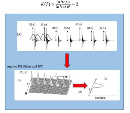
Figure 2 - Spectrum data analysis. a) Time trace signal, b) The FIR filters bank, c) The outcome of the Spectral Kurtosis analysis.
