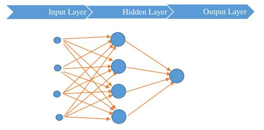
Figure 7 - Denotes a typical feed-forward neural network with a single hidden layer.
