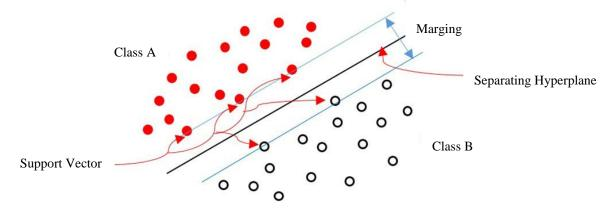
Figure 4 - Support Vector Machine (SVM) structure.
