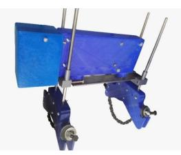
Figure 2: Designed and developed measurement system for shaft alignment.
